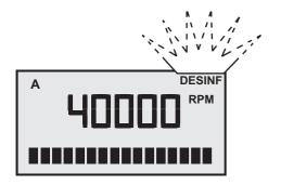
If the message DESINF starts flashing on the dentist element display during treatment, then 1 liter of DEN-TOSEPT P should be refilled not later than the end of the treatment day.
