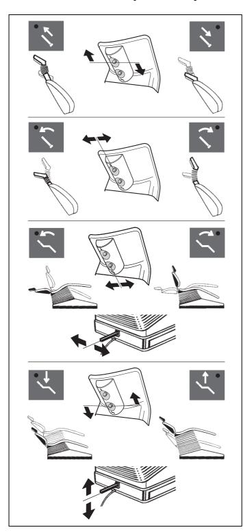
The keys located on the right key block of the dentist element control panel can be used to trigger the different chair movements manually.
