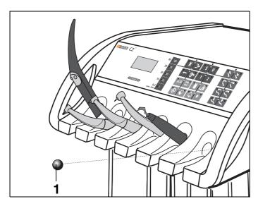
A ball stopper for an unoccupied instrument holder is enclosed with the dentist element.
