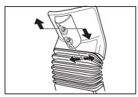
By actuating the 4-way switch on a motor-adjustable headrest in any direction.
