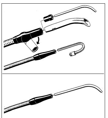
The vacuum system is switched on after a suction hose is removed from the holder.
