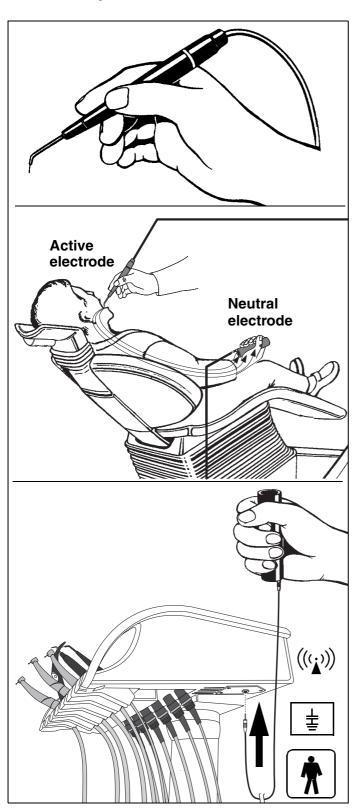
The electrosurgical handpiece is used for electrotomy (cutting), coagulation and desiccation in biterminal technique.
