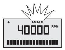
The message AMALG appears on the display if the amalgam rotor needs replacement, i.e., when having reached a filling level of 95% (see instructions "Care and Cleaning by the Practice Team").
