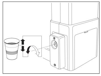
The filling level of the tumbler can be preset with the knob on the base of the water unit (foot end).
