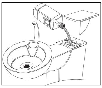
Remove the cover behind the cuspidor and fill in 1 liter of DENTOSEPT P.
