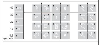
With this foot switch, all functions can be controlled using the entire pedal surface for hands-free working. However, it is also possible to work manually by key operation.
