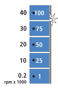
The intensity is set by briefly (< 0.5s) activating the quick setting keys in increments of 1 / 25 / 50 / 75 / 100.
