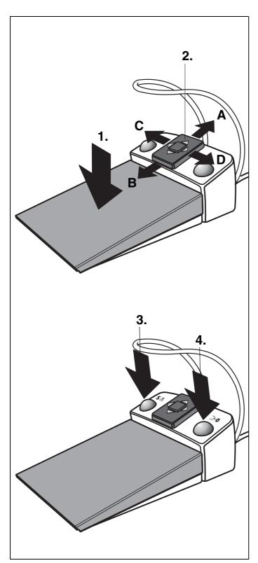
This foot switch allows you to work with both hands free using the cursor control or manually by key operation.
